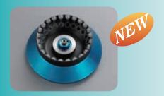
Shield rotor can attain processing of 24 x 1.5/2.0 mL tubes — MA-2724 Rotor 0.2-mL PCR tubes may also be centrifuged.
